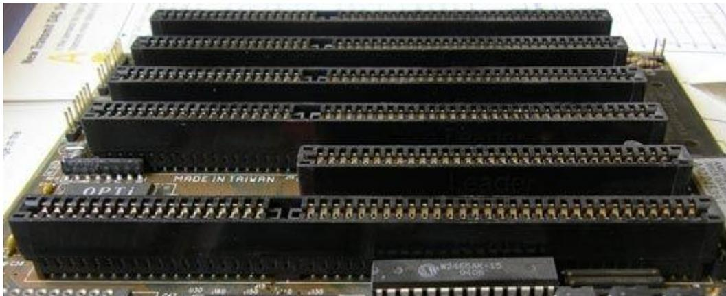
Figure 2. ISA bus: 4 x 16-bit and 1 x 8-bit ports.
