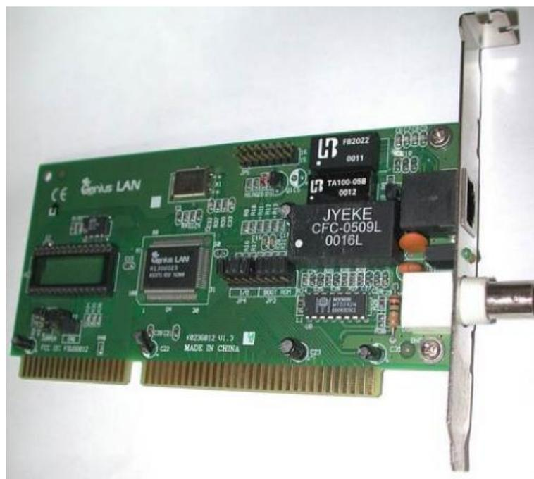
Figure 1. ISA bus-based AUI port network card.
