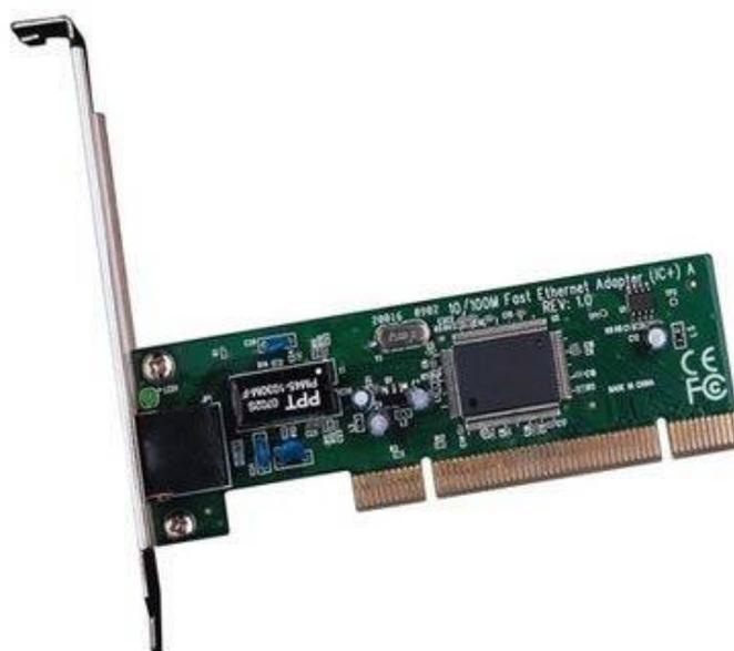
Figure 3. PCI port network card.
