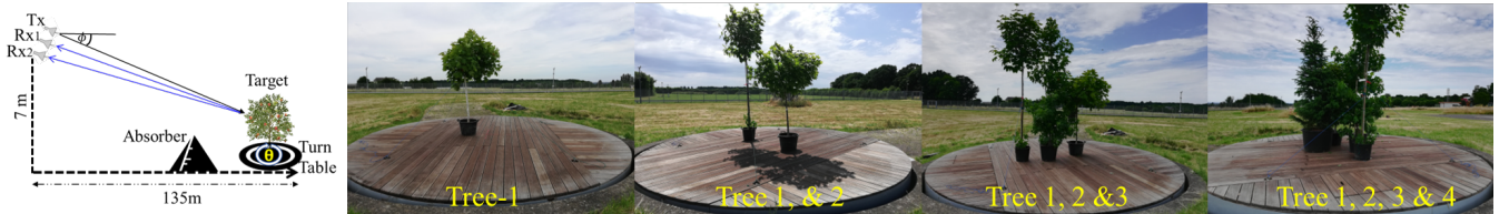
Fig. 1. ISAR COBRA radar ( f_c = 9.6 GHz) system is deployed to scan rotating trees with different arrangements of tree types.
