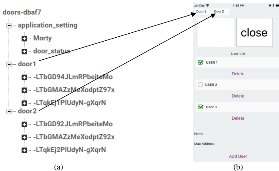
Figure 12. Two-door locks system using two sub-databases (a) firebase database and (b) Door Lock App
