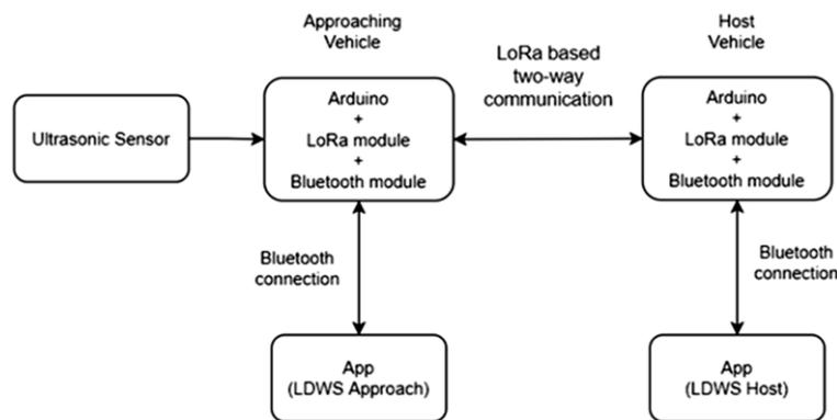
Figure 4. System architecture
