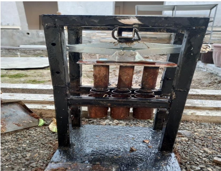
pic1. General view of the stand for making cups from waste.
