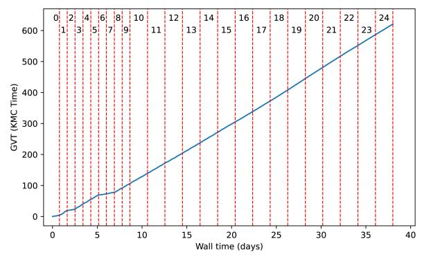
Figure 5: Global virtual time (GVT) plotted against wall time for our Brusselator simulation with 625 processors. Red, dashed lines are used to indicate where the simulation was paused and later restarted. The numbers on the top represent the simulation restart index of each chunk.
