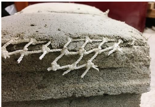
a) Overlay reinforced with #21 nylon fishing net and bonded onto concrete masonry substrate
