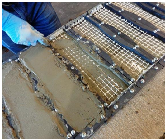
a) Casting of fishing net-reinforced cementitious overlay specimens
