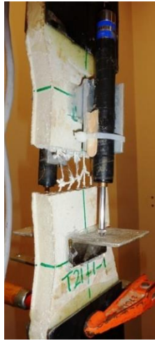
a) Typical failure mode of fishing-net reinforced overlay
