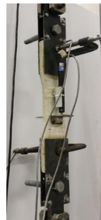
c) Close-up of dogbone specimen
