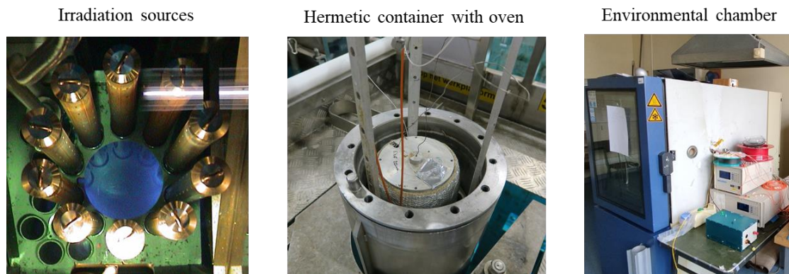
Figure 1. Photographs of the experimental facilities: the irradiation sources (left), the hermetic container for irradiation of the sample (center), and the environmental chamber for climatic experiments (right).
