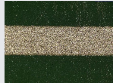
Fig. 4. Image from Leica DMS1000 stereo-microscope. Ag NP printed electrode with optimal process parameters at 200°C/30 min.
