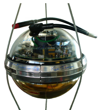
Figure 3.11: Photo of an assembled IceCube DOM. Picture courtesy of the IceCube Collaboration.
