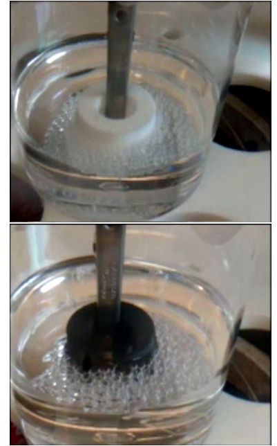
Figure E.2: Picture of bubble formation under samples that were evacuated over ten minutes at 10 mBar. The photograph on the top is of a plain PA12 sample, and the bottom is of a painted one.
