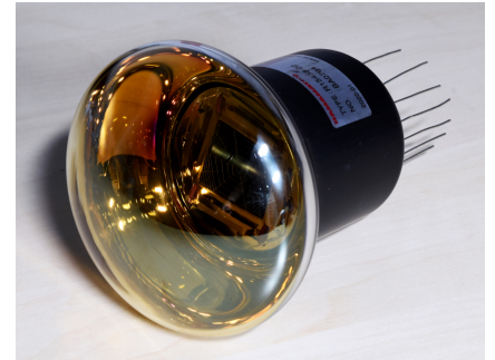
Figure 4.3: Picture of the Hamamatsu R15458-02 PMT. Published in [110].
