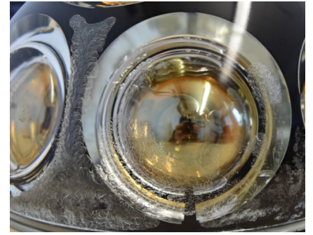
Figure 10.10: Aftermath of cooling one of the first mechanical prototype. The gel breaks and delaminates as a result of thermal stress.
