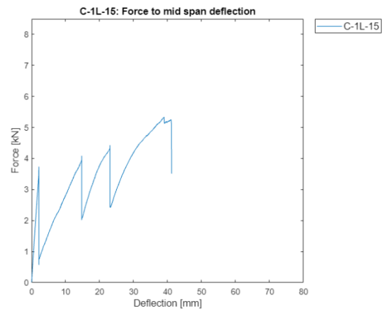
Figure 9: Load-deflection curve of specimen C-1L-15 with 1 coated CFT layer and 15 mm cover thickness
