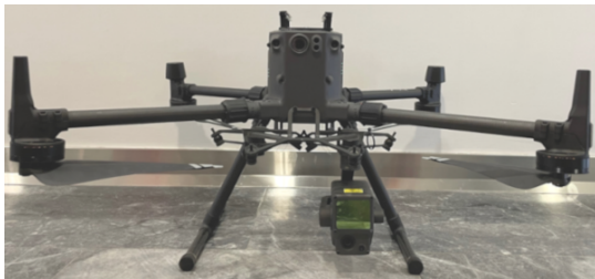
Fig. 2: UAV and LiDAR sensor used for acquiring data
