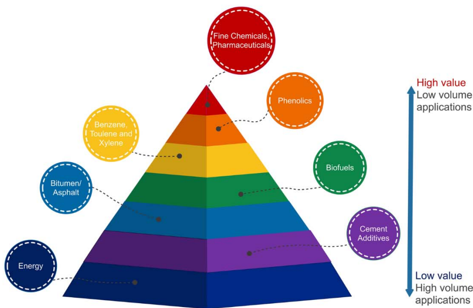
Fig. 3 Potential lignin applications and relative values of different product classes. Adapted from [243]
