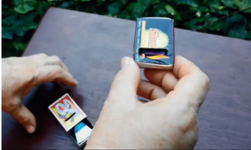
Fig. 11. Matchbox spectroscope. With a piece of CD.
