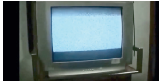
Fig. 7. Detection of the microwave background with a TV.
