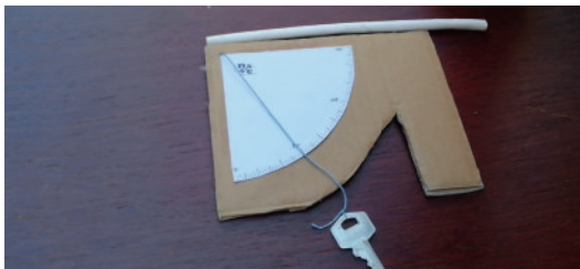
Fig. 3. Gun dial, to measure vertical angles.
