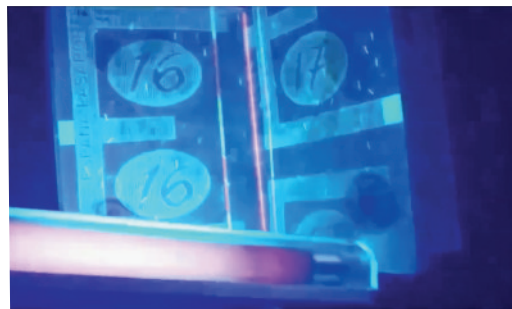
Fig. 12. The UV light from a counterfeit banknote detector shows things that are not normally seen.
