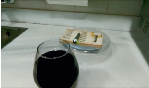
Fig. 9 Simulation of a gravitational lens with a cup. The distance from the flashlight should be similar to the diameter of the cup.
