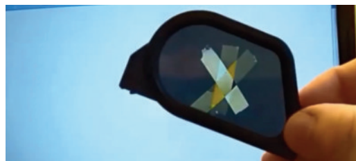
Fig. 5. Polarized light from a computer screen, with several layers of adhesive tape.
