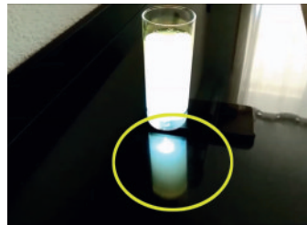
Fig. 15. The light coming from the sides is bluish. That is why the daytime sky is blue.
