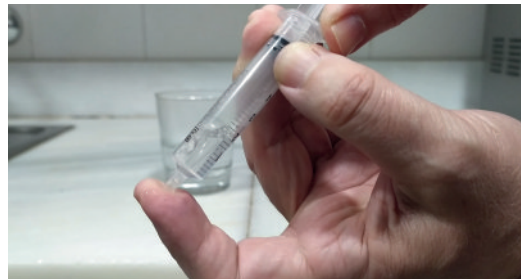
Fig. 4. Decreasing the pressure, the water boils.
