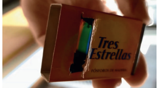
Fig. 12. Through the slit, the spectrum of light can be seen.
