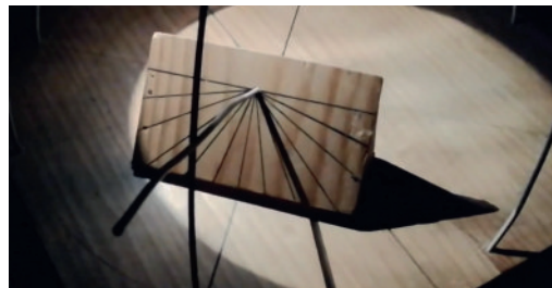
Fig. 8. How an equatorial sundial works.
