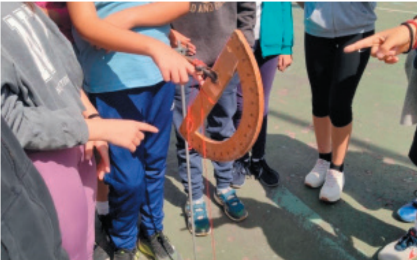
Fig. 9: With a semicircle oriented towards the sun, we can obtain its height (1st Experimental Junior High School of Maroussi, Greece) (Credit: V. Petridou)
