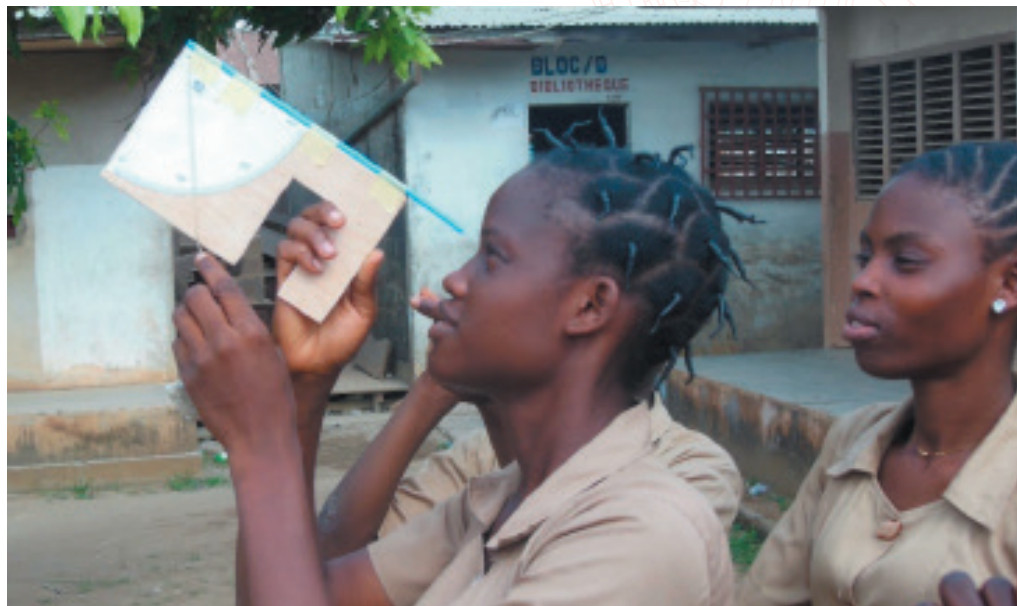
Fig. 15: Practicing with the dial to read the angle obtained. Terrestrial applications allow calculation of the height of a building or a mountain. (CEG ALPASSA, Porto-Novo, Benin) (Credit: PA. Ahanhanzo).
