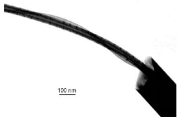
Figure 30-69: The first inorganic nanotubes in Ljubljana: a pair of WS 2 nanotubes grow from the inside of the micro-tube. A narrow tube with a diameter of 18 nm is wound sufficiently evenly around a thicker tube of diameter 40 nm. The mating of both tubes can be explained by the formation of intermediate surfaces between the crystalline nets of the two tubes. Contact between pipes is possible only at points where the arrangement and orientation of the walls are in accordance with the P63 / mmc spatial group (photo: Maja Remškar).
