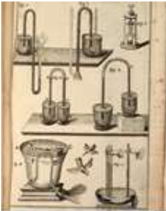
Figure 6-118: Huygens' siphons in Figure 4 from the second part of the Ferrari's philosophy with physics (Ferrari da Monza, 1754, 2: Tab 5 and p. 2: 88).
