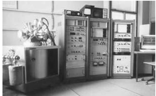
Figure 13-6: Auger's spectroscop of PHI, SAM, 545A of Physical Electronics Inc. Minnesota in the surface analysis laboratory at the Department of Surface Technology and Optoelectronics of the IJS (until 2003 Institute for Surface Technology and Optoelectronics - ITPO) 1501
