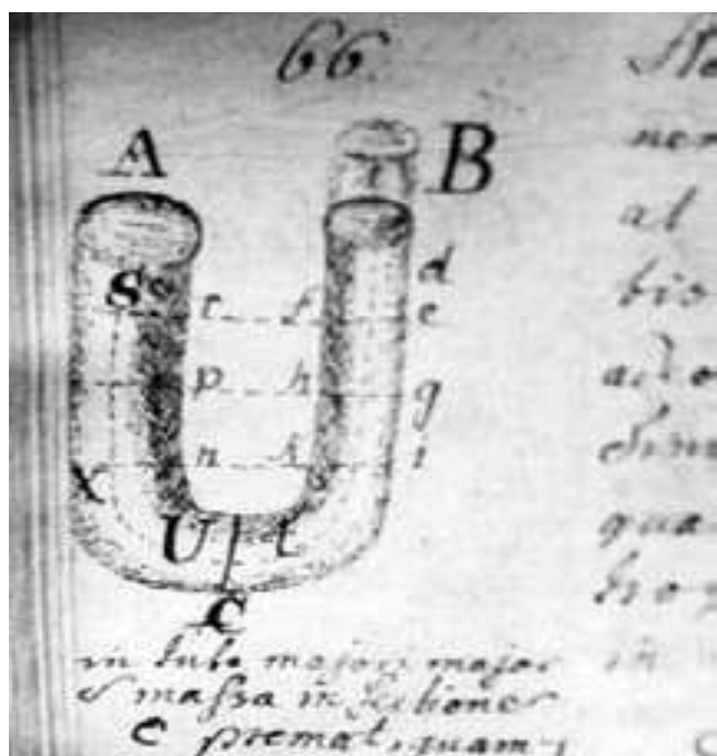
Figure 6-33: Hieber's sketch of the equilibrium in a liquid as an introduction to the description of vacuum pumps (Hieber, 1797, 66); F
