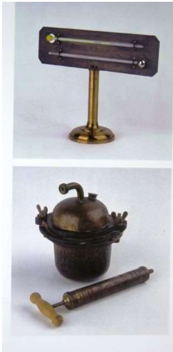
Figure 6-218:Maximal-minimal thermometer and Papin's Pressure cooker with a pump at Koper Grammar school.
