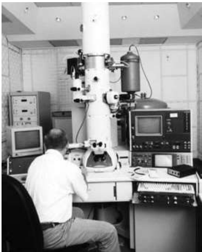
Figure 25-5: An analytical transmission electron microscope Jeol JEM-2010F at IJS
