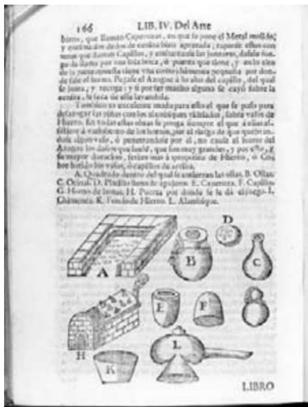
Figure 14-6: Parts of Barba's vessels needed for his amalgamation painted in his Metallurgy from the Sumitomo's Library (Barba, 1729, 166).
