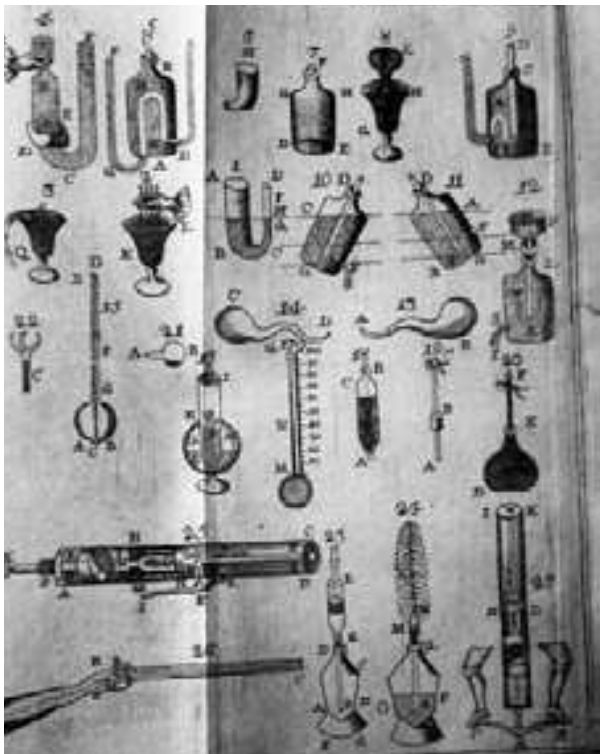
Figure 6-159: Air rifle and barometers by Donatus in Ljubljana Franciscans' library (Donatus Hofmann, 1754, table of figures 3).
