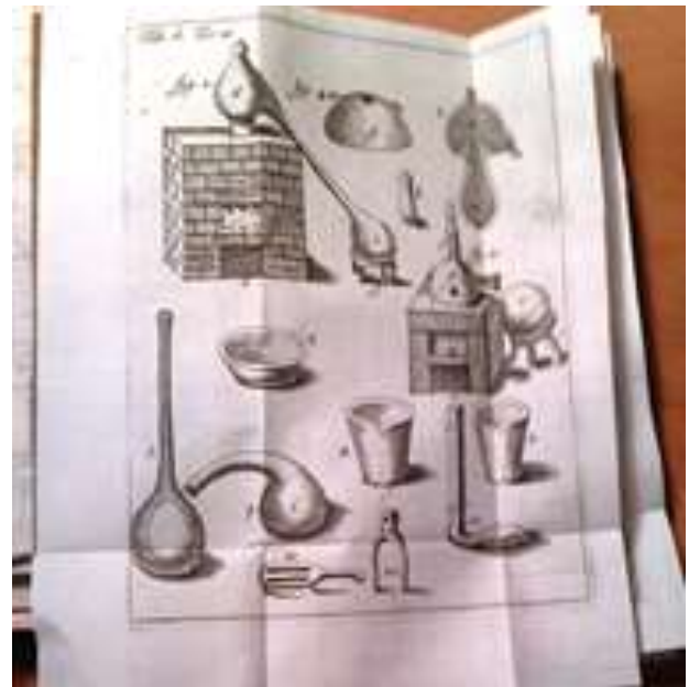
Figure 6-100: Pourchot's table of pictures presenting the distillation (Pourchot, 1730, 2: Table 6)
