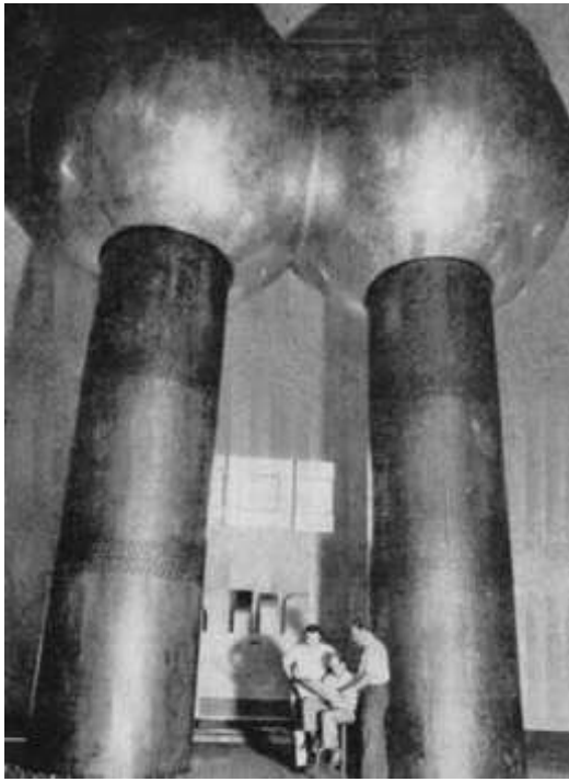
Figure 26-3: Van de Graaff generator at MIT, below three Van de Graaff's co-workers 2944
