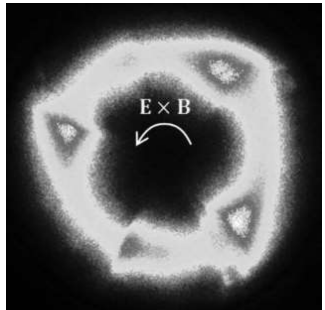
Figure 18-13: Magnetron plasma shot with a fast camera (exposure time 10 ns, author of the image: dr Matjaž Panjan)
