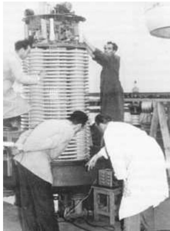
Figure 26-5: Electrostatic Van de Graaff generator for two million volts with an open boiler and a high-voltage electrode at the IJS in Ljubljana 2946
