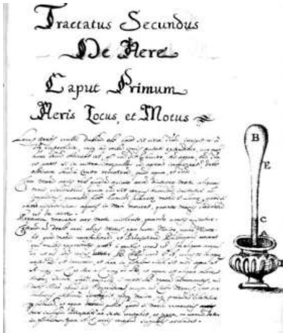
Figure 4-3: Paolitto vacuum barometer from the second half of the 17th century (Paolitto, after 1657, folio 15v, with the permission of the curator of the history of science at the University of Oklahoma, Dr. Kerry Magruder)
