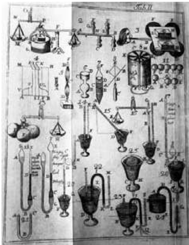
Figure 6-160: Donatus' barometers and siphons in Ljubljana Franciscan library (Donatus Hofmann, 1754, Table of images 2); F.
