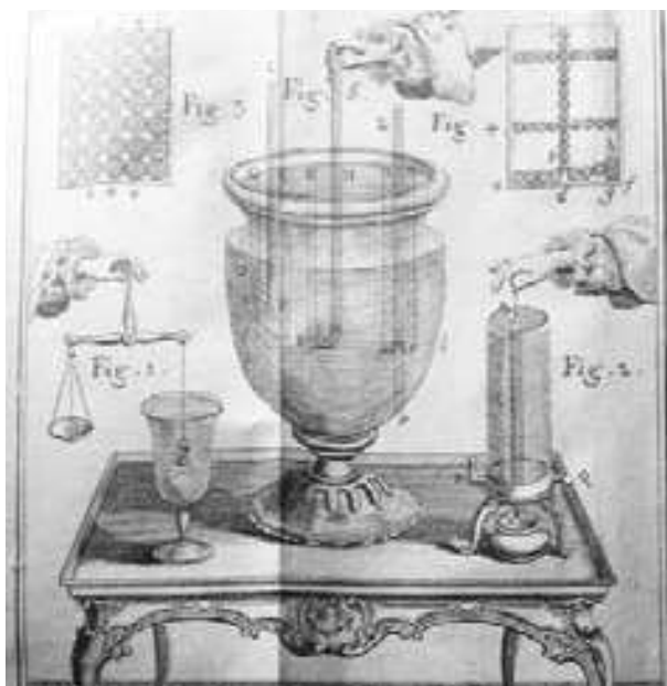
Figure 6-134: Nollet's vacuum experiment with barometers and air gun at Ljubljana Franciscans' library (Nollet, 1751, table of figures 3, lection 7 of second part)
