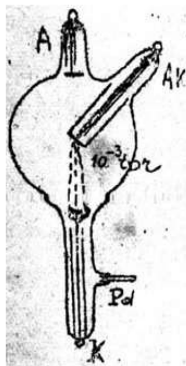
Figure 30-3: The vacuum cathode ray tube in first Slovenian university textbook of physics (Peterlin, 1940, p. 261 and Appendix 1).
