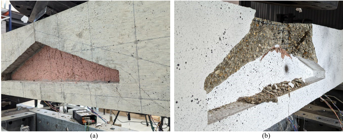
Figure 4: Failure mode of the functionally graded TRC beam: (a) Visible bending cracks in the bottom tie and shear crack originating from the support inclined in direction of the centre void (b) Concrete compression failure at the top of the beam and visible from the back side of the specimen.
