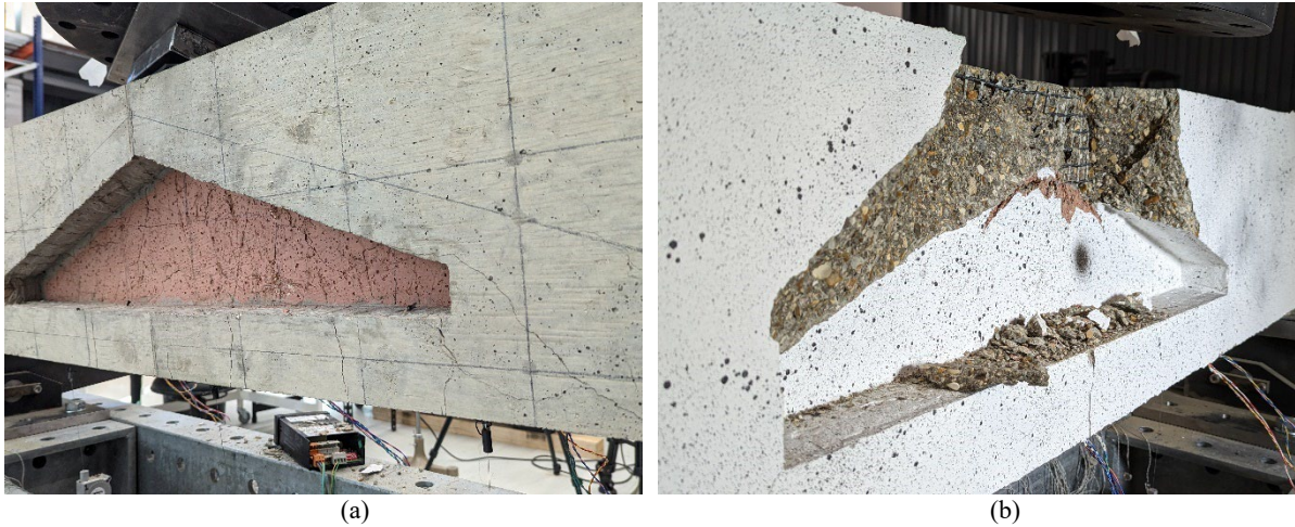
Figure 4: Failure mode of the functionally graded TRC beam: (a) Visible bending cracks at the bottom tie and shear crack originating from the support inclined in direction of the centre void (b) Concrete compression failure at the top visible at the back side of the specimen.
