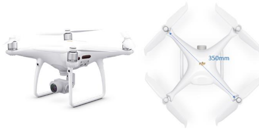
Figure 4-14. Dimension of DJI Phantom 4 Pro v2.0
