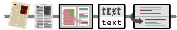
Fig. 1: Main components of a typical OCR workflow. From left to right: original image, Preprocessing, Layout Analysis (regions & lines), Text Recognition, Post-Correction
