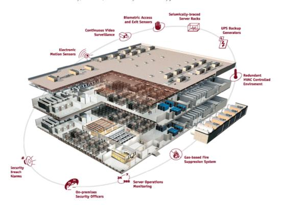
Figure 1: Shows an example of services considered critical for a general-purpose datacentre. Adapted from "The Exodus 1999 Annual Report", http://archive.icann.org/en/tlds/i1/REGOP/Exodus%20proposal.htm
