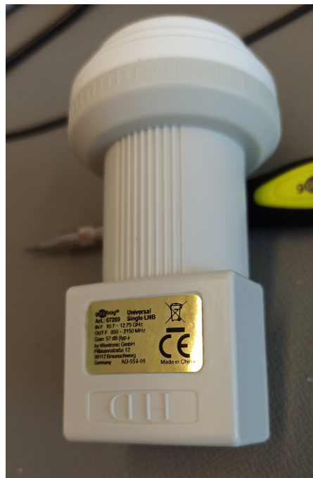
Figure 1: Unmodified Goobay 67269 LNB
