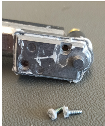
Figure 3: Removal of the PCB housing screws
