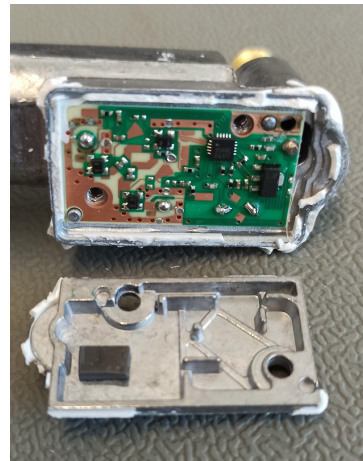
Figure 4: Metal cover of the LNB removed
