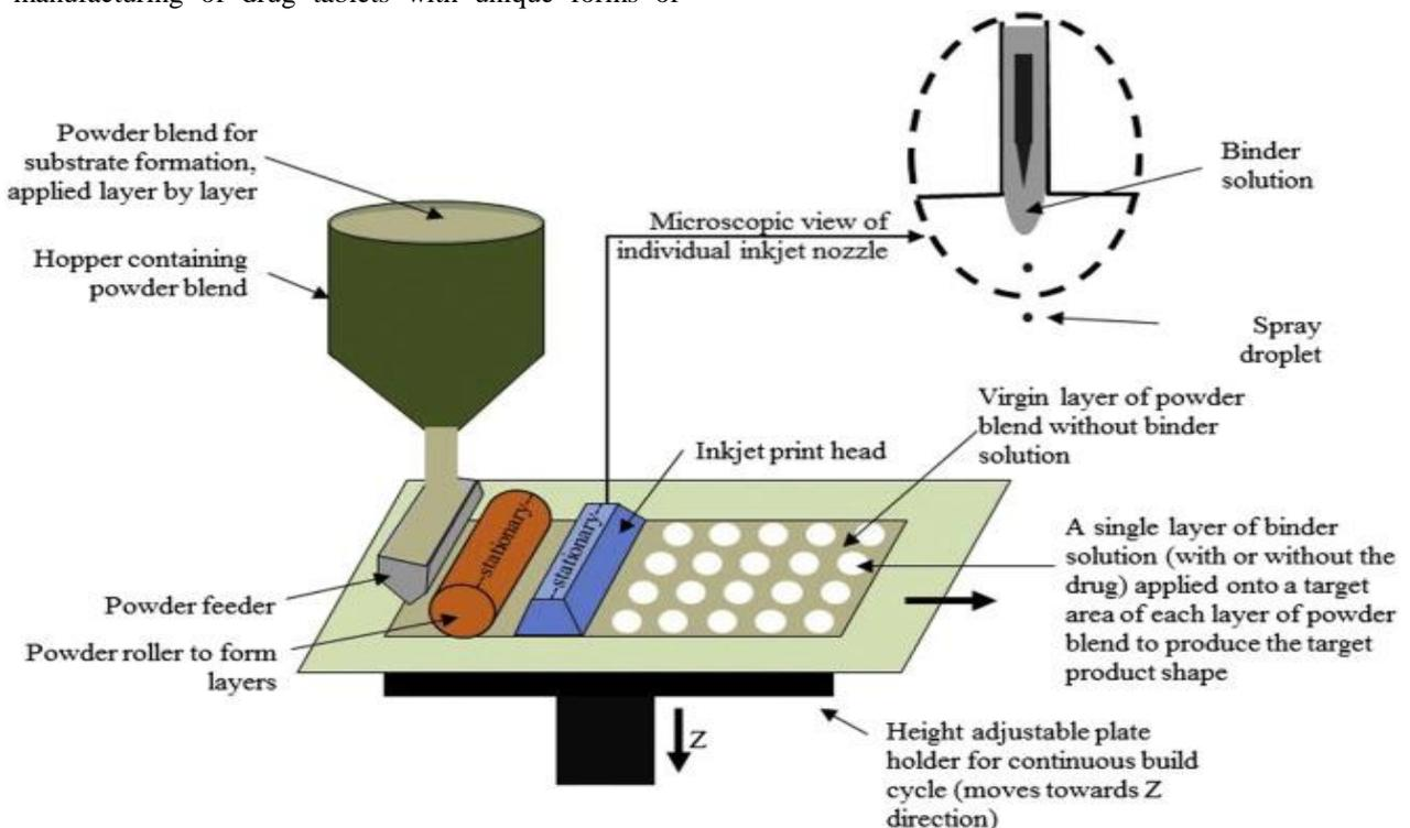
Fig. 7. Process of making drug items with the help of the 3D printing technology [16]
