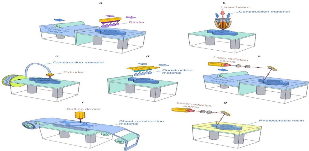
Fig. 3. Different types of 3D printing are currently in the utilization [9]
