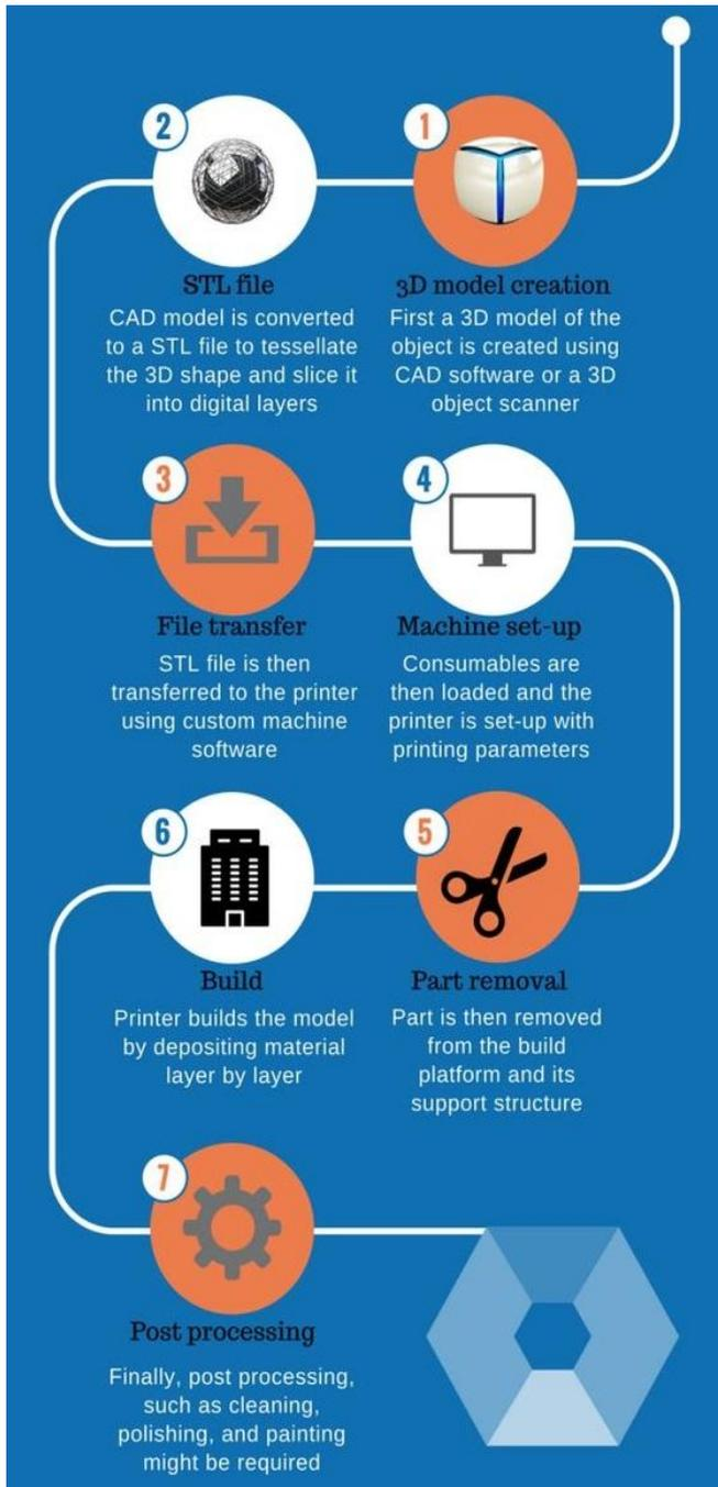
Fig. 2. The procedure of 3D printing [4]
