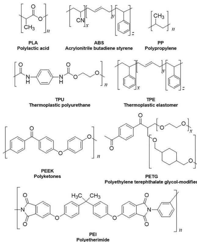
**Fig. 1. The organic structure of the polymers utilized as raw materials for 3D printing [2]**
