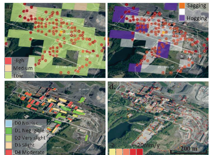
Fig. 3. Hazard zones (after [6]): a. Deflection b. Horizontal strain c. Hazard based on relative rotation for concrete buildings (after [5]) d. Measurement points with LOS displacement velocity. Lazy mine, Ostrava-Karvina POHO
