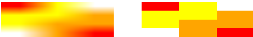
Figure 13.9. Example bitmaps drawn with rasterImage , with (left) and without (right) colour interpolation.
