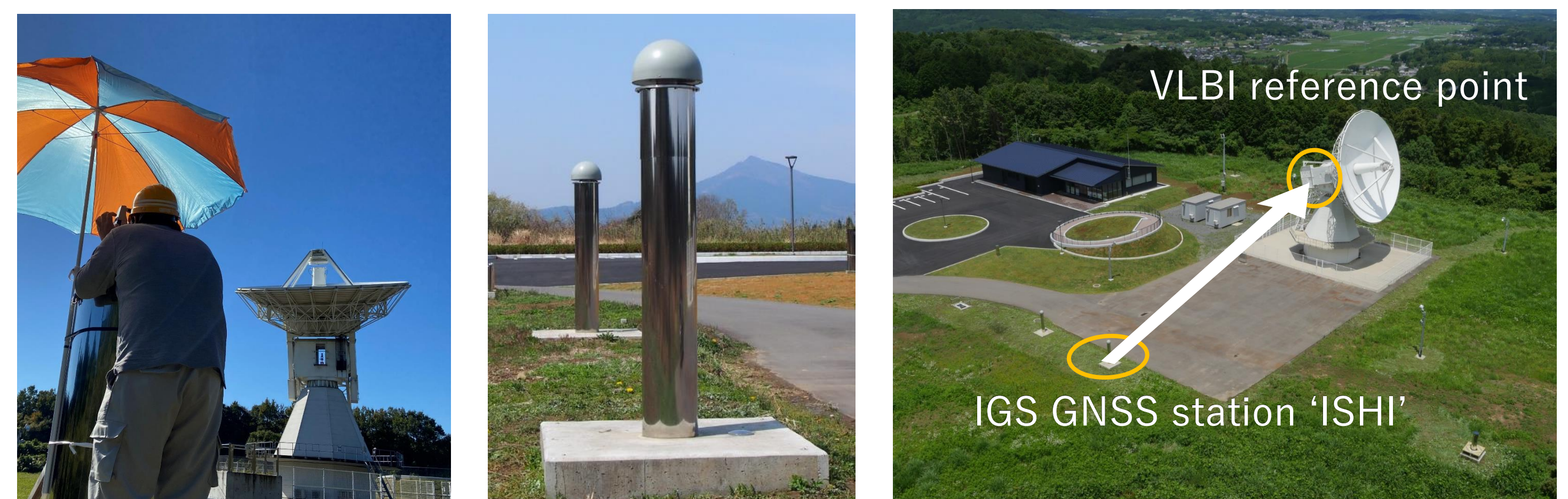
Fig. 6: (Left) Measuring the positions of the mirror installed in the AZ cabin from the pillar using the TS. (Middle) GNSS station called ISHI, which is registered as an IGS station. (Right) VLBI-GNSS local-tie vector.
