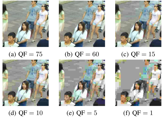
Fig. 2: Sample 200 \times 200 pixel image patch taken from the Shanghai Tech Part B dataset [4], after being compressed with a varying QF.
