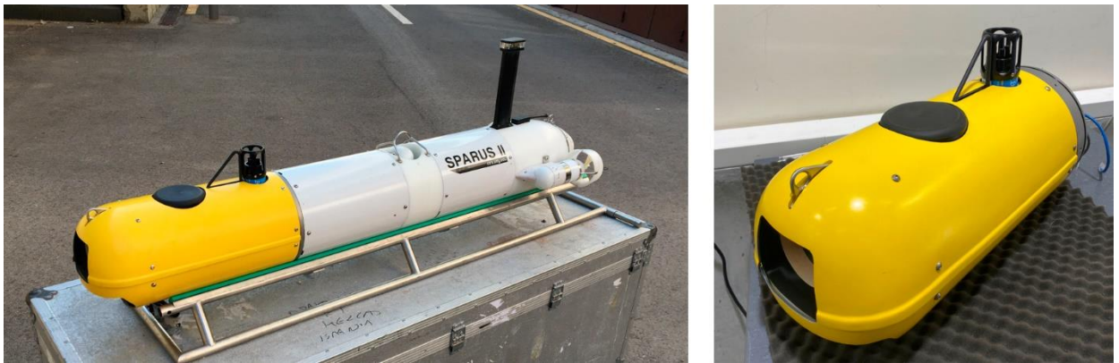
Figure 2-2: Payload for the docking task installed on the Sparus II AUV.
