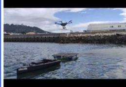
Autonomous landing of RAVEN on NEST trailed to NAUTILUS ( https://youtu.be/8pUfmgZT9w )
