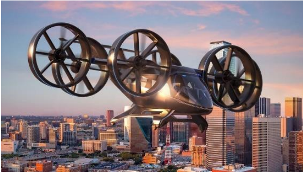
Figure 12. Bell Nexus 6HX with ducted rotors
