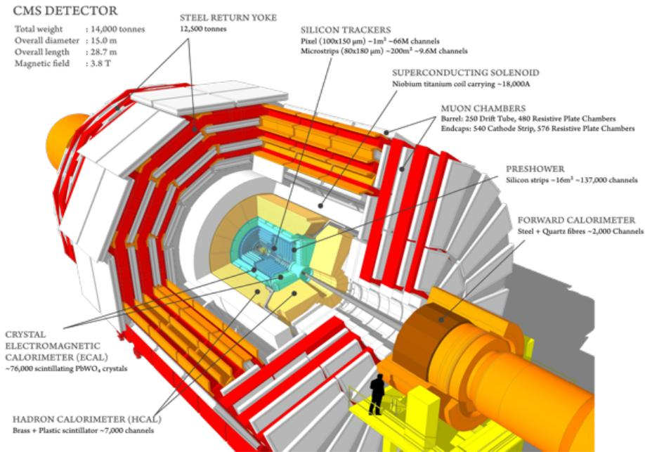
Figure 2: The CMS Experiment at CERN LHC.
