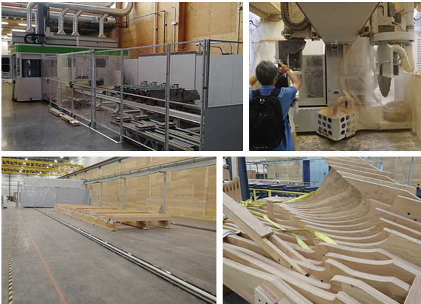
Figure 9.15 A computer numerical control machine used for machining of complex wooden elements used in timber structure.
