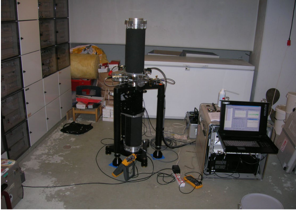
Figure 2. The FG5#216 from the ECGS at the absolute gravity station of Nuuk. The gravity benchmark 78801 is visible on the left side of the FG5. Due its proximity to the electrical cabinet, it was not possible to set-up the FG5 on top of it.
