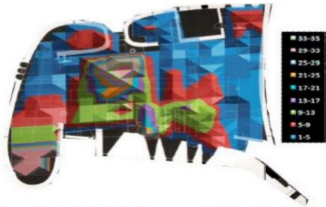
Fig.17 Daylight factor in open door environment:0.6%, 0.23% ratio of uniformity (on site measurements)
