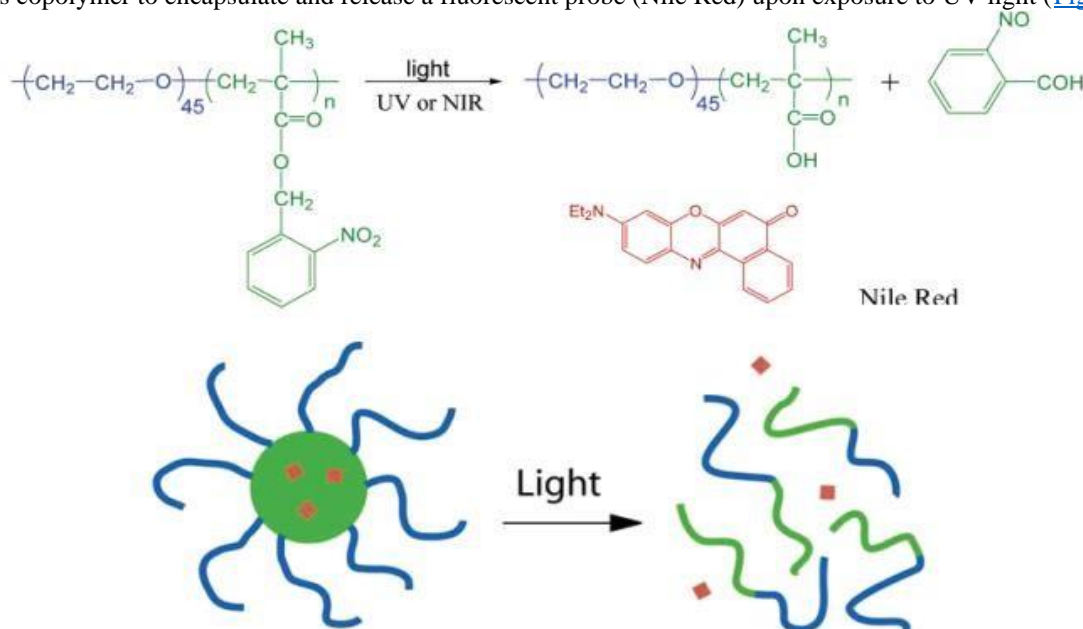
Figure 24: (a) Irradiation of a PEO-b-PNBM copolymer (b) Schematic representation of the destruction of a micelle and release of an active ingredient under the effect of irradiation
