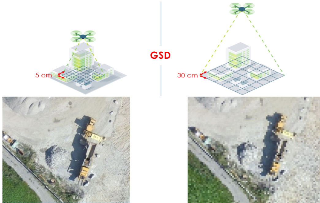
Fig. 9: Correlation between flight height and GSD (modified from PIX4D, 2019)
