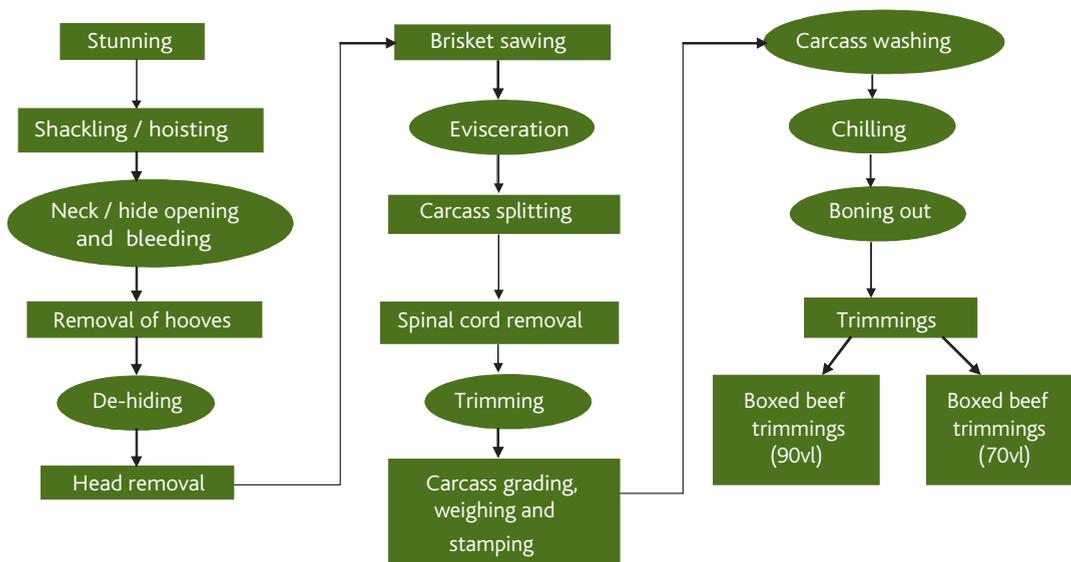
The model assumed that contaminated hide and gut contents were the main vector for cross contamination to carcasses at the hide removal stage and at evisceration cross contamination factors from hide to carcass and from rumen contents to carcass were created (Figure 6, 7) based on Irish surveillance data for the pathogen on bovine hide (O'Brien *et al.*, 2005a) and on beef carcasses (McEvoy *et al.*, 2003; Carney *et al.*, 2006).
