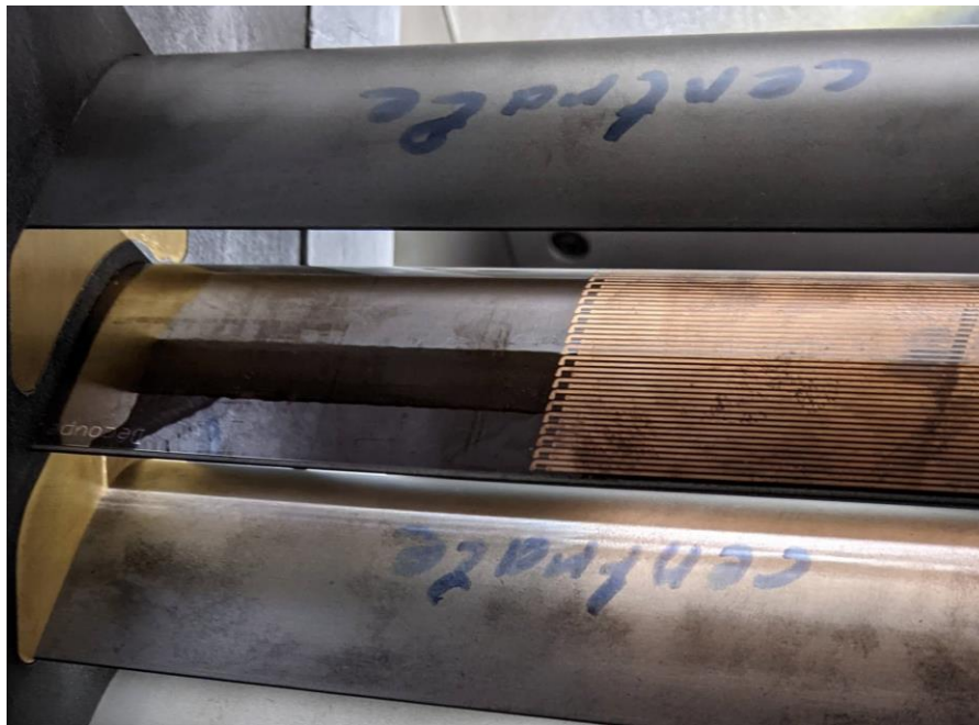
Figure 2.26: Blade instrumented with fast-response hot-film sensors mounted in the SPLEEN cascade.
