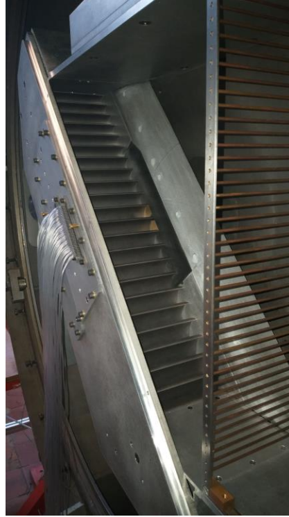
Figure 3.9: Turbulence grid installation in the wind tunnel
