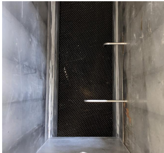
Figure 2.6: Location of the pitot tubes at the entrance of the test section.
