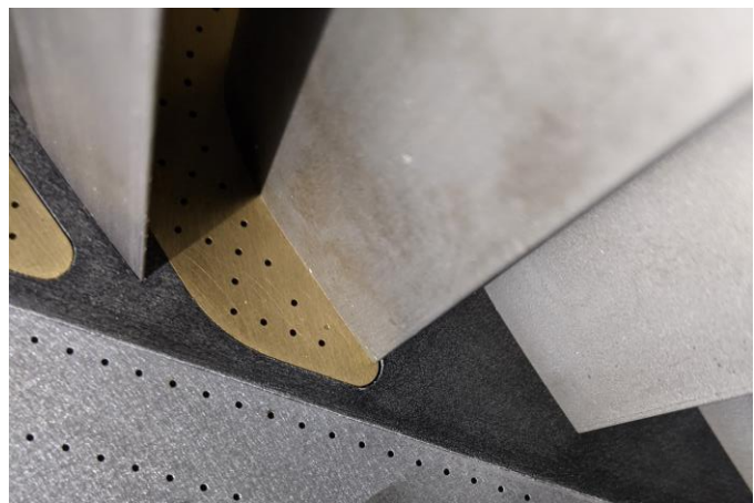
Figure 3.5: Integration of the smooth and instrumented inserts into the SPLEEN cascade
