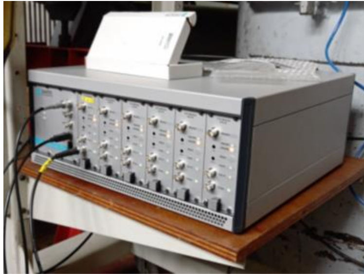
Figure 2.36: Dantec Dynamic Streamline Pro Constant Temperature Anemometer.
