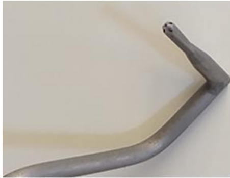
Figure 2.16: Cobra five holes probe P-PNEU-C5HP-01
