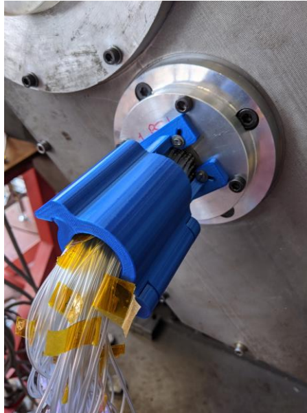
Figure 2.34: Pneumatic connector and 3D printed support.
