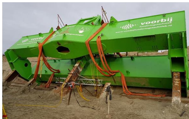
Figure 28 Load frame used for MV Pile tests
