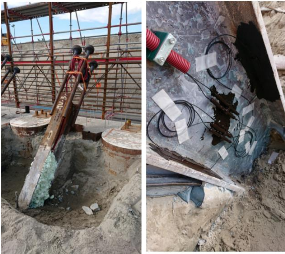
Figure 31 FBG gauges on MV Piles (Schouten 2020)
