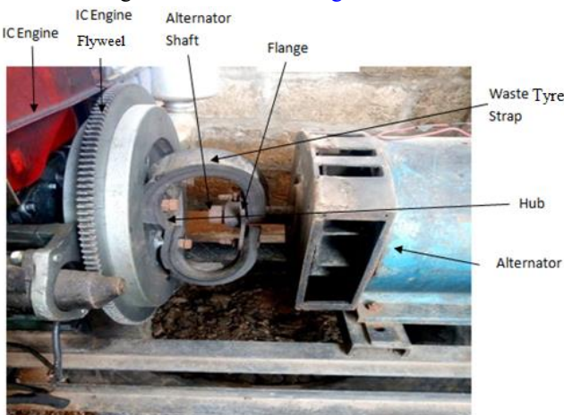
Fig. 2 Waste tyre coupling system test arrangement
