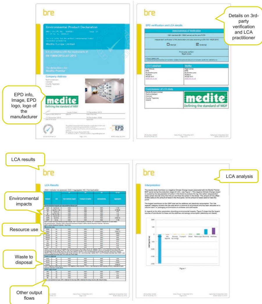
Fig. 9.5 Examples of environmental product declarations (EPD) for wood products including a Medite MDF product and a Protec treated timber landscaping product.
