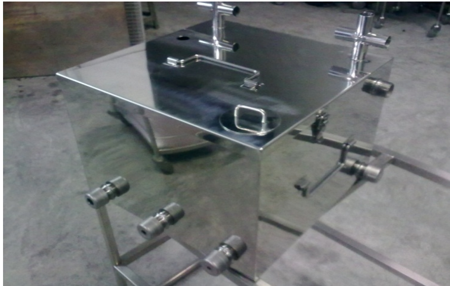
Fig. 4. Water collection tank
