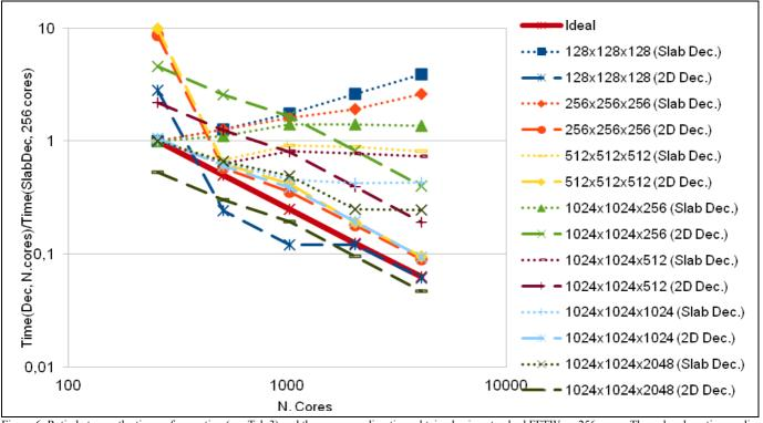
Figure 6: Ratio between the times of execution (see Tab.3) and the corresponding time obtained using standard FFTW on 256 cores. The red and continuous line is the ideal scalability line. Dotted lines are related to standard FFTW efficiency, whereas dashed lines are related to 2D<sup>3</sup> efficiency.
