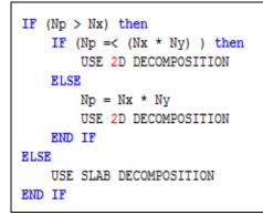
Algorithm 2: The first simple algorithm used to switch from standard slab to 2D domain decomposition
