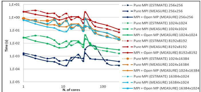
Figure 3: Plot of the execution times reported in Table 1, using MPI communications (both FFTW\_MEASURE and FFTW\_ESTIMATE cases), and hybrid MPI+OpenMP communications (only FFTW\_MEASURE case).
