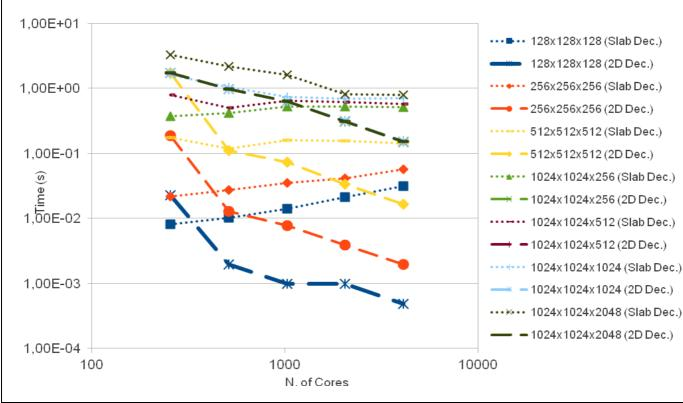
Figure 5:Plot of the execution times shown in Table 3. Dotted lines are referred to Slab Decomposition, whereas dashed lines to 2D Decomposition.
