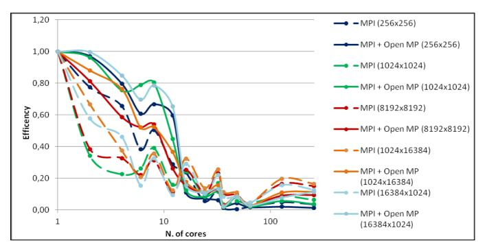
Figure 4: Efficiency obtained during the scalability test of Figure 3
