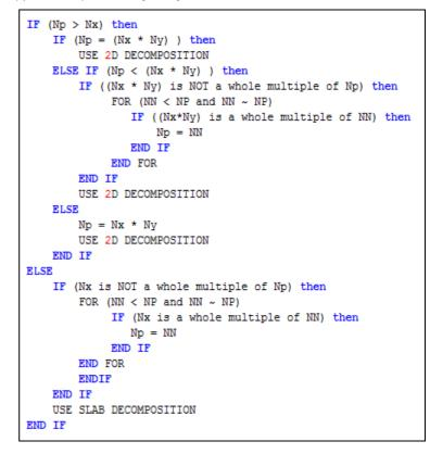
Algorithm 3: An improved version of *Algorithm 2*, that includes also the main features of *Algorithm 1*.
