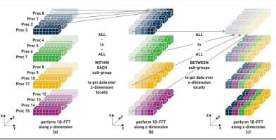
this algorithm pays a higher cost in terms of MPIFigure 2: 2D Decomposition of a 3D DFT. The array was divided between 16 MPI process. communications, but it ensures higher scalability. From (8).
