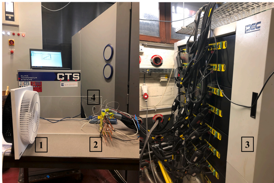
Fig. 2. The picture of the experimental system (1) Cooling fan; (2) LTO cell and SHCS; (3) PEC® battery tester (4) Personal computer and, Datalogger.
