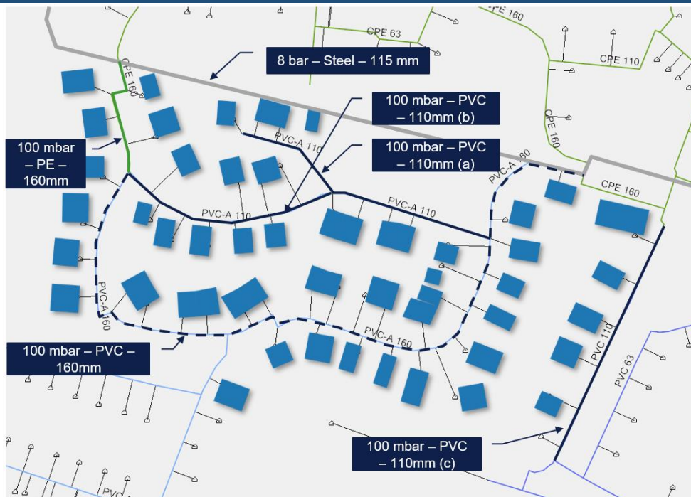
Figure 25 Overview of houses and the distribution grid in the case study.
