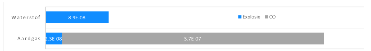
Figure 12 Comparing individual risk of hydrogen and natural gas for explosions due to a leak in the indoor installation and CO poisoning.
