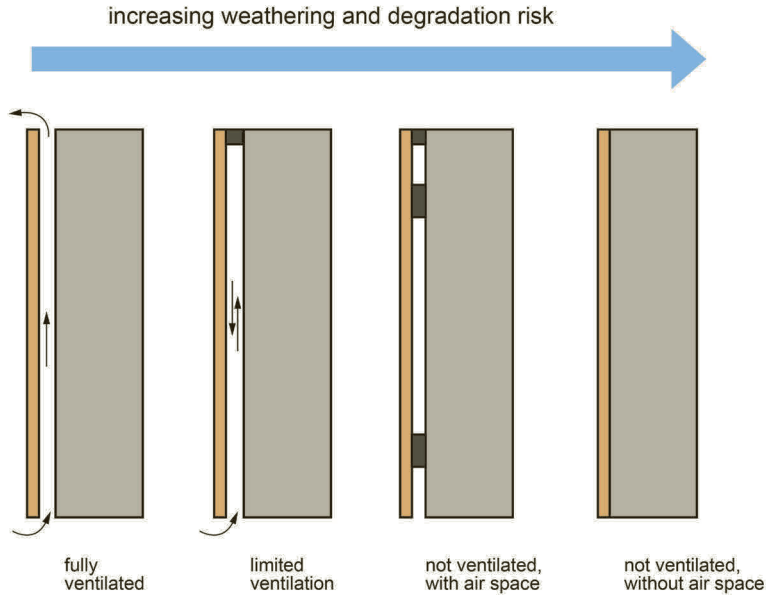
Figure 1.77 The way in which ventilation can alter the performance of timber cladding (modified from Isaksson et al., 2015).
