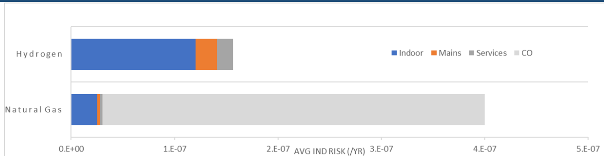
Figure 38 Average location-based risk per home in the case study for hydrogen and natural gas
