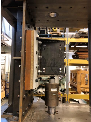
c) full-scale connection tested in strong-axis bending
