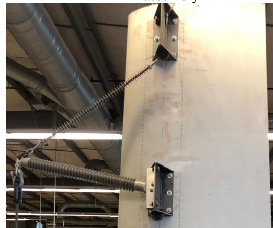
e) braced-line post assembly tested
