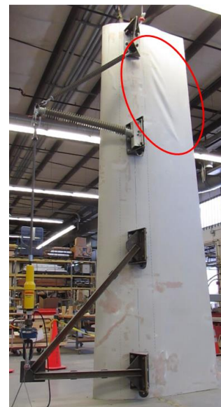
d) buckling of the wind blade shell under loading
