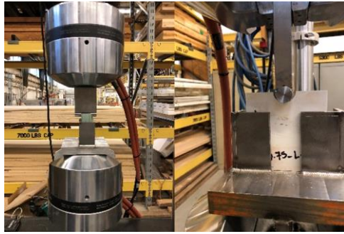
a) specimen tested in pin-bearing
