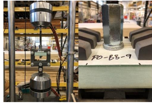
b) specimen tested in pullout
