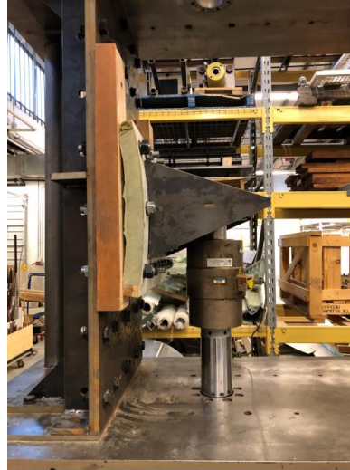
d) full-scale connection tested in weak-axis bending
