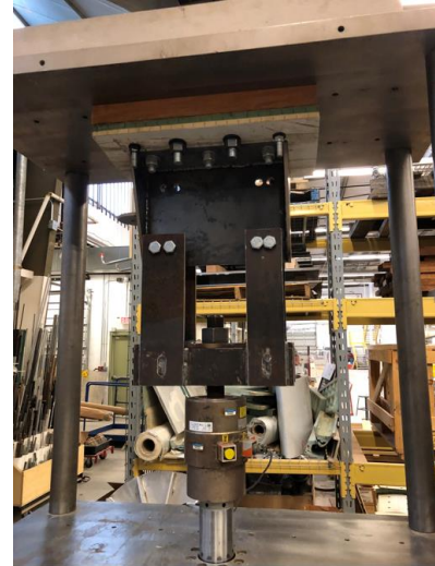
e) full-scale connection tested in pullout
