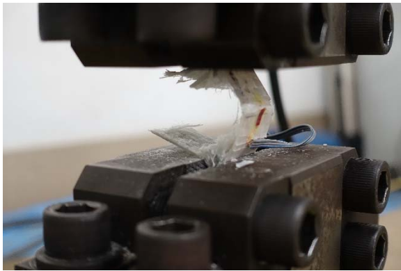
Figure 8 Compressive fatigue failure
