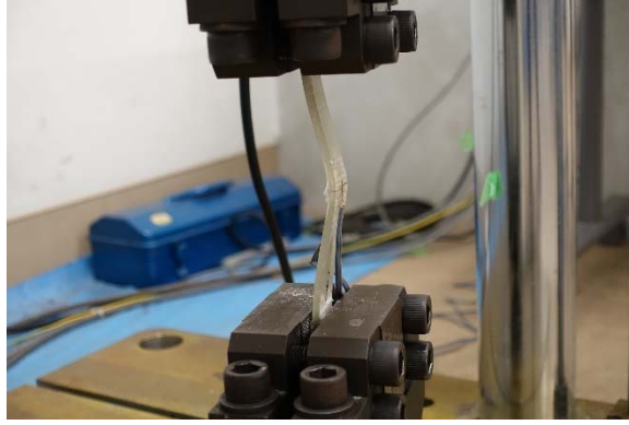
Figure 5 Buckling mode of 250-mm-long specimen
