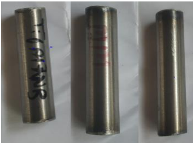
Fig. 1. Ti-6Al-7Nb alloy Test Specimens
